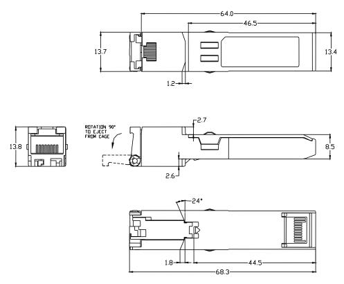
Figure 2. Mechanical Dimensions of Transceiver
