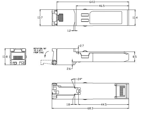
Figure 2. Mechanical Dimensions of Transceiver
