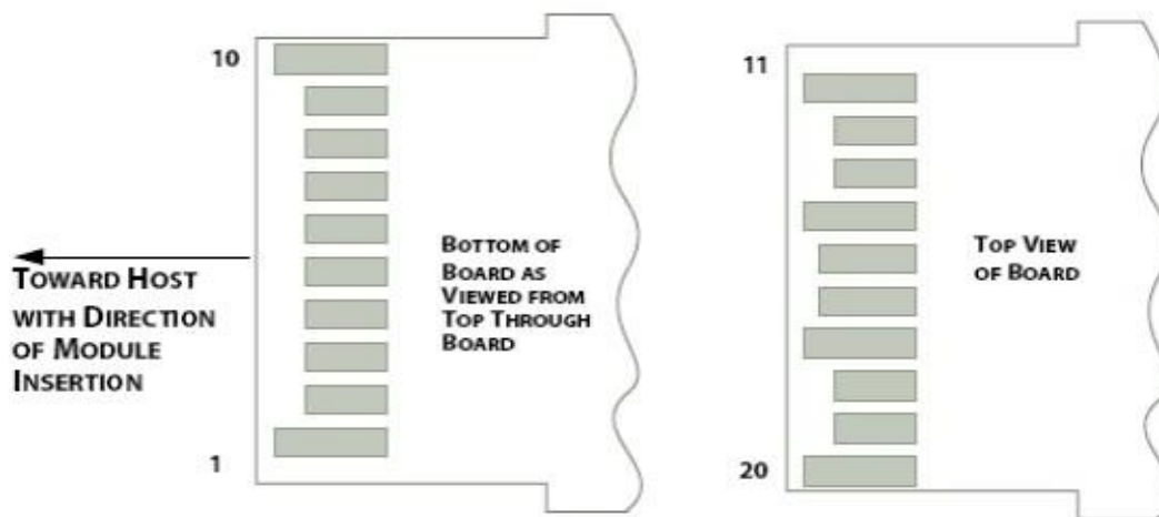
Figure 3. SFP28 Module Contact Assignment
